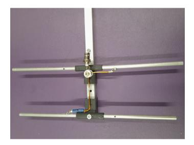
The 3D printed parts that holds the elements were modified to the spacing between the elements. A slot was also added to where the phasing line is down the centre of the boom.
