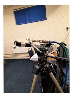
Getting back to the HB9CV antennas, this has been a long term project and when it is finalised and all dimensions tested, we will 3D print the final brackets in a single piece. The final design will then be available for all to make, if required, free on request.
