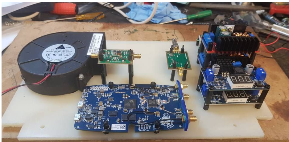
Left to right: Fan with 80mm hole under it. The small PCB is the PA Driver board below it is the now naked Pluto. To the left is the Bias-T then the 4 PSUs for +28, +18, +12 and +5vs
