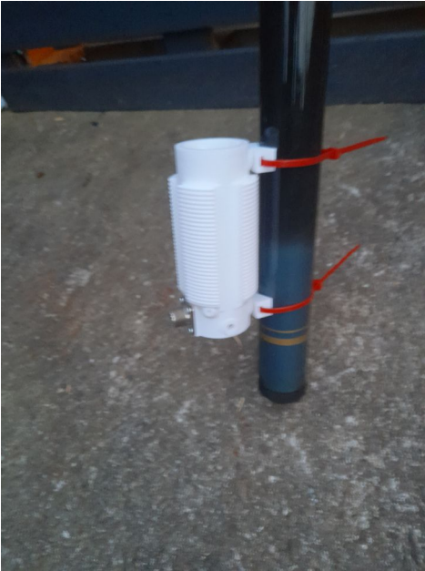
A Coil former 3d printed ready for winding
