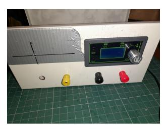
On the left you see the PSU in the making. The outputs are entirely up to you. It could be just the Black & Red binding posts for the variable voltage.
